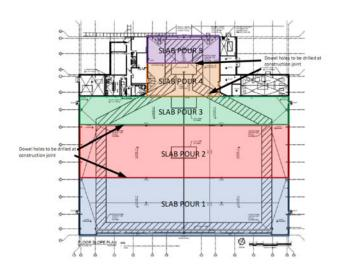
While this plan for placing the slabs certainly saves some time by eliminating the number of construction joints with dowels, it created many headaches for the project team when it came to determining effective finishing methods. The 75 feet sections are much wider than most slab pours that Kinsley Construction typically deals with on other projects. To complete the process, some of the intended finishing techniques must be modified and potentially compromised.
